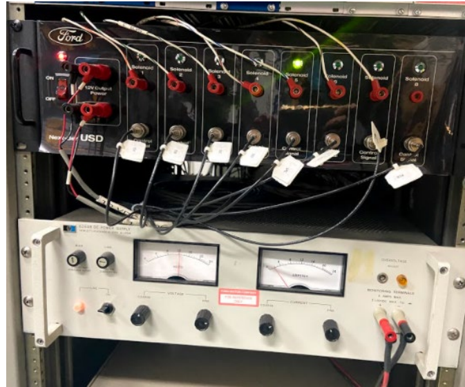
Figure 26: Solenoid controller and power supply.
