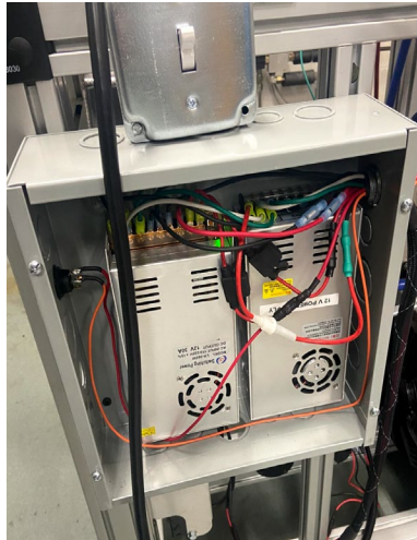
Figure 50: Remove enclosure cover to provide airflow to power supplies
