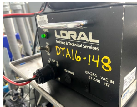
Figure 28: Power supply for transmission
