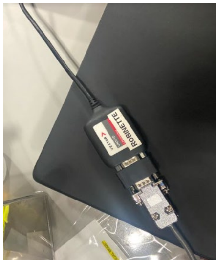
Figure 77: Vector tool connection to USB to computer and to DB9 cable
