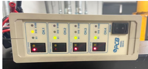
Figure 27: Signal conditioner for AC One Tach
