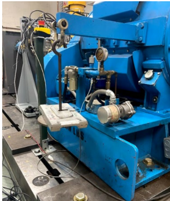
Figure 84: Calibration weight application on AC Dyno
