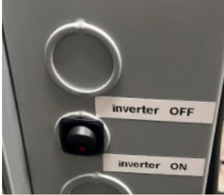
Figure 83: Power cycle the inverter to establish new motor position
