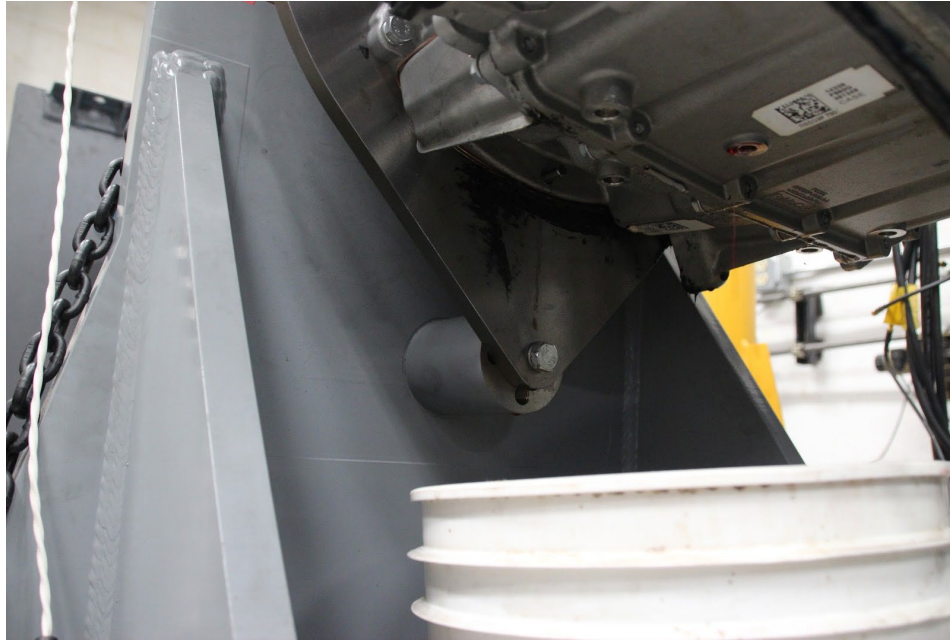
Figure 141: \frac{3}{4} " bolt removal on bottom of headstand
