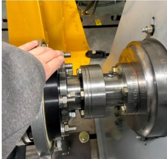
Figure 29: Checking free rotation of input motor shaft
