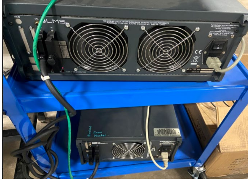
Figure 54: Turn on the DAQ systems. Turn on the Master DAQ (top) before turning on the smaller DAQ (bottom)
