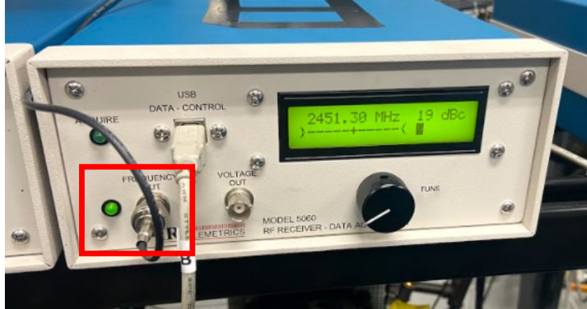
Figure 95: Receiver box “Frequency Out” port to send marker signal to TOMBox
